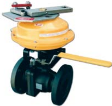
The MT (mid-torque) fusible link assembly incorporates the valve handle to allow for normal operation even with the valve armed.
